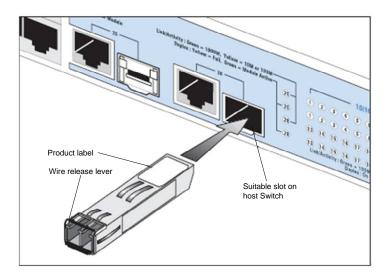
2) Gently slide the transceiver into the SFP slot until it clicks into place.
